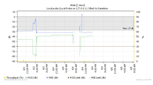
For an example of a link that is outside of tolerance, see this graph:
