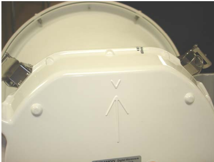
Figure 11 HP ODU Vertical Polarization
