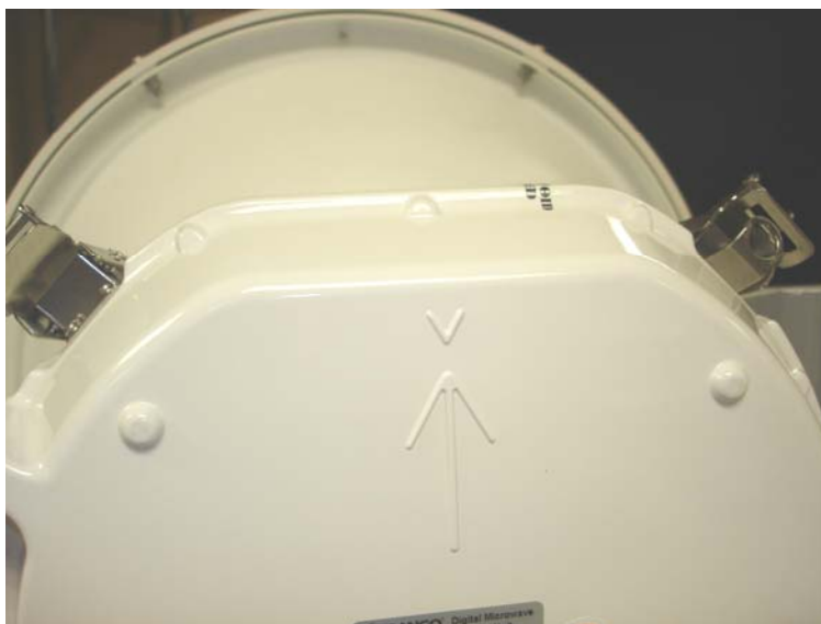
Figure 10 HP ODU Vertical Polarization
