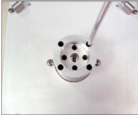
Figure 23: Installing twist transition on 1+1 coupler
