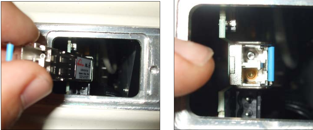
Figure 15: SFP Module installation
