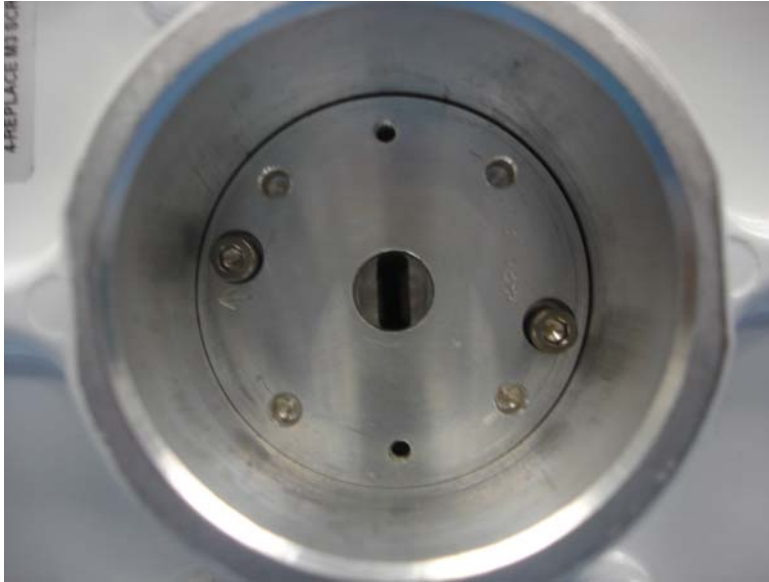
Step 2d Completed HORIZONTAL Polarization Antenna Port
