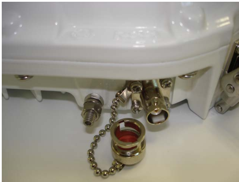
Figure 39 BNC Connector for RSSI Voltage
