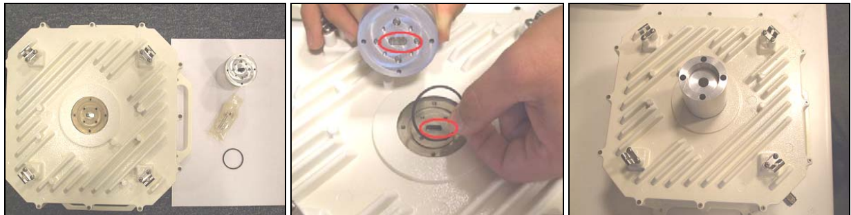
Figure 13: Waveguide transition installation.
