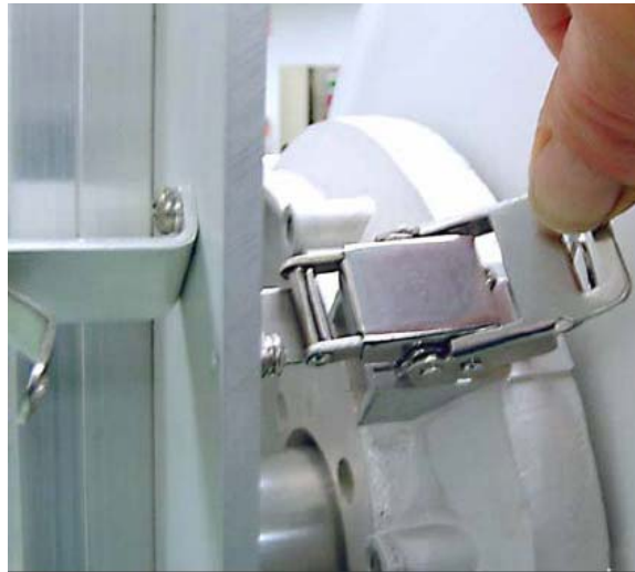
Figure 17: 1+1 Coupler and latches
