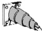
Figure 23: Weather Proofing of cable
