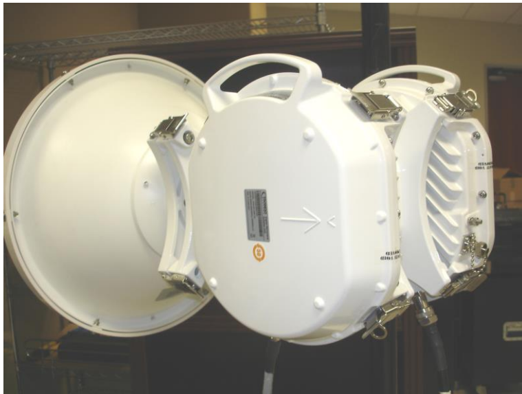
Figure 30 ODUs on SMC combiner (1+1)
