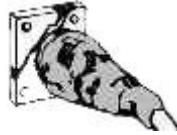
Figure 51: Complete weather proofing of cable
