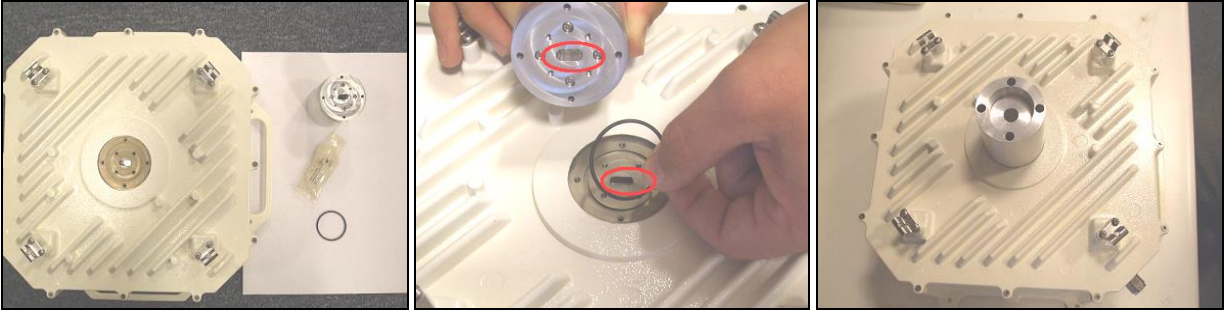
Figure 42: Waveguide transition installation for SP ODU.
