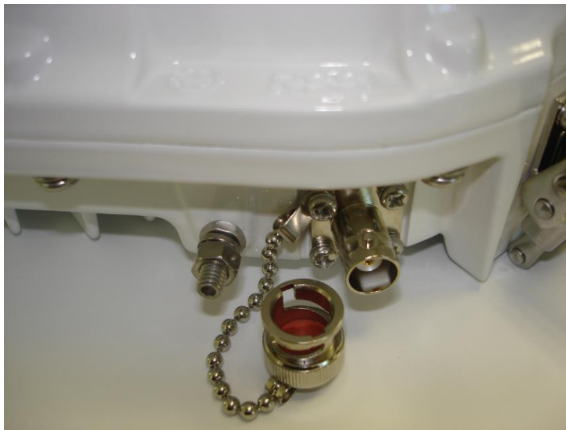
Figure 39 BNC Connector for RSSI Voltage
